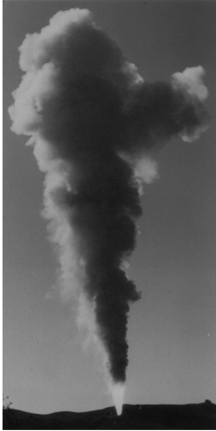
Figure 1.1: Photograph of the turbulent plume from the ground test of a Titan IV rocket motor. The nozzle exit diameter is 3m., the estimated plume height is 1,500m., and the estimated Reynolds number is 200 \times 10^6 . For more details see Mungal and Hollingsworth (1989). Permission to be obtained.
